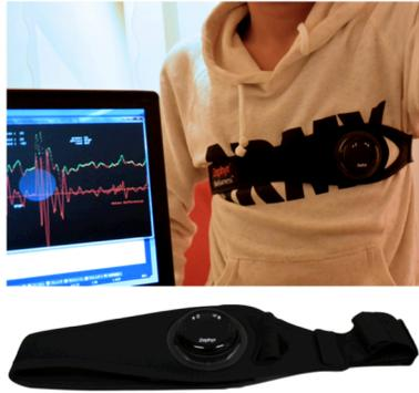
**Figure 3:** The Zephyr BioHarness™ 3 and our software in use by a user. Normally the device is worn under ones clothes.
